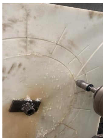
Figure 1. Example of a polyamide part machined on a CNC milling machine
