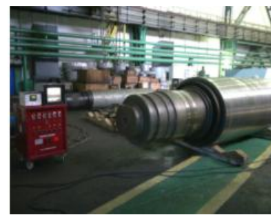
Figure 10 Heat treatment station
