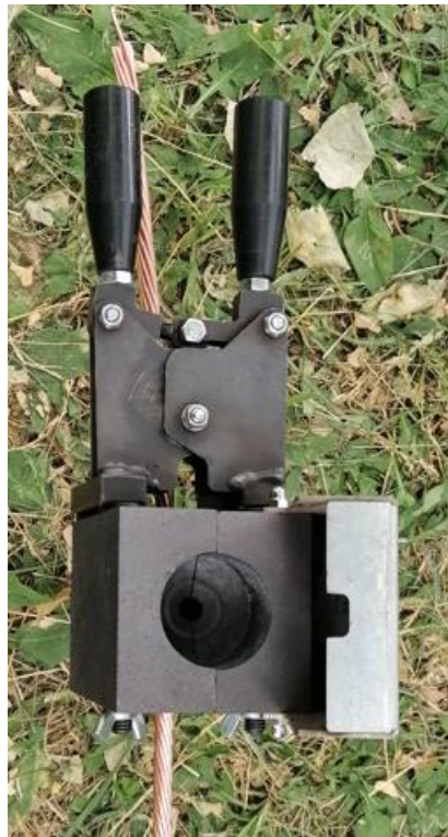
Figure 1. Mold used for aluminothermic welding of earthing sockets
