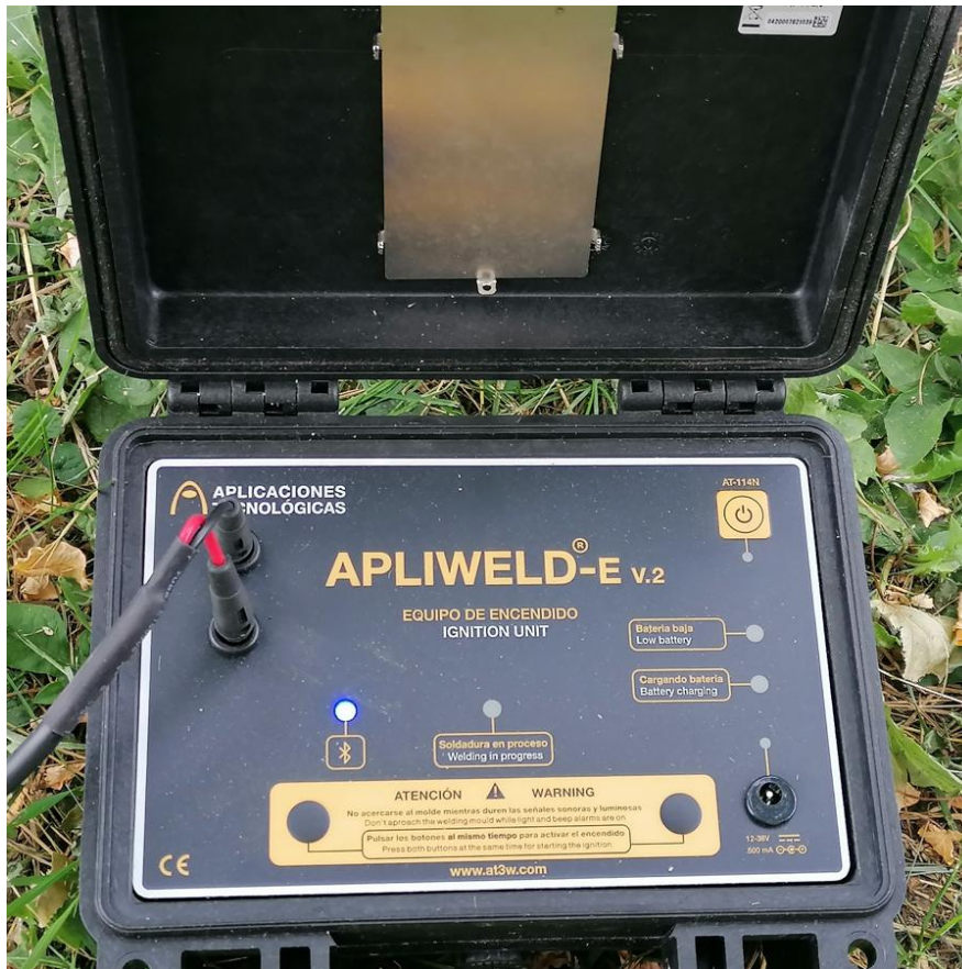
Figure 2. Reaction initiation device for aluminothermic welding
