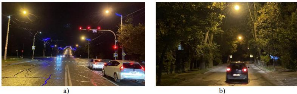
Figure 5. a) Location of bilateral lighting system; b) Location of suspended/central lighting system [3, p. 427].
