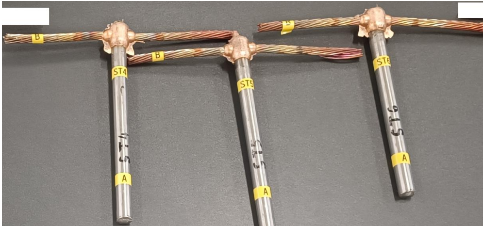
Figure 4. ST4, ST5 and ST6 welded joints between copper sheet and stainless steel electrode
