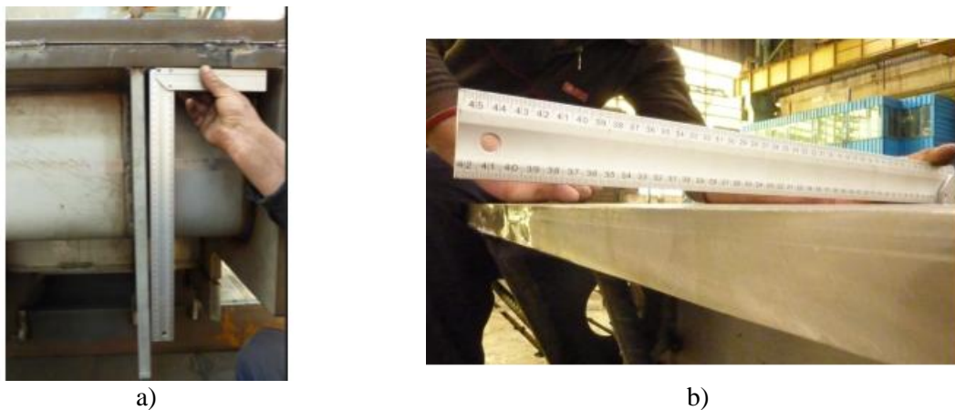
Figure 9 – Position deviations/ from the plastic deformation technological process
