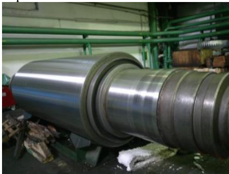
Figure 14. LBC cylinder with reconditioned spindle
