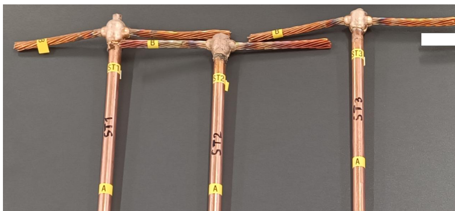
Figure 3. Welded joints ST1, ST2 and ST3 between copper sheet and copper electrode
