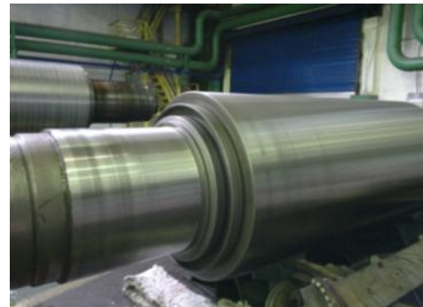
Figure 14. LBC cylinder with reconditioned spindle
